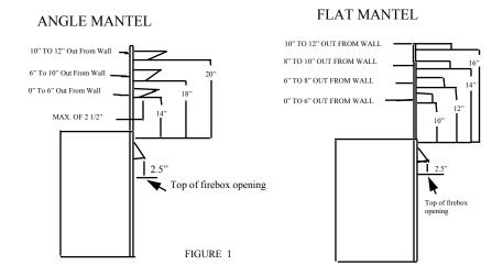
Mantel minimum clearances for a listed Zero Clearance Firebox or a Masonry Fireplace.
